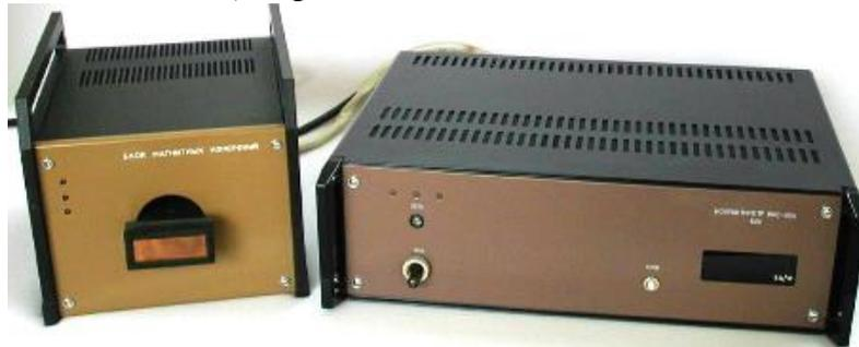
Fig. 6. VKS-968 type structurescope (coercimeter) for coercive force evaluation in open magnetic circuit: magnetizing-demagnetizing unit (left); measuring unit (right).
