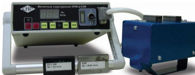
Fig. 1. Magnetic structurescope (coercimeter) KRM-Ts with calibration blocks.
