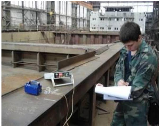
*Fig. 14. The process of coercive force measurements along the "river-sea" type ship coaming.*
