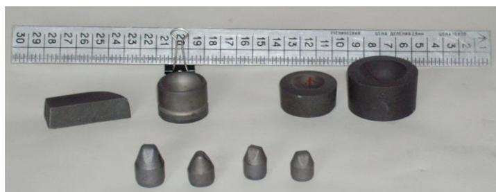
Fig. 15. Hard alloys products evaluated by coercive force measurements in open magnetic circuit.
