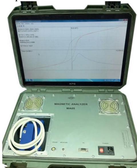
Fig. 4. Magnetic analyzer MA-05 for multiparameter measurements.
